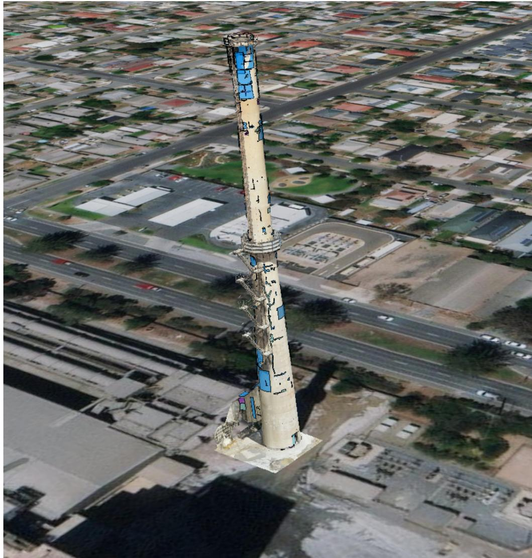
Ingenia have added visual inspection to the services delivered from the UAV. The obvious advantages with visual inspection done in this method are the speed in which an inspection can be done and the safety risk mitigation through not having personnel in elevated platforms or on scaffolding and via rope access. The cost benefits far outweigh the alternative methods of visual inspection.
